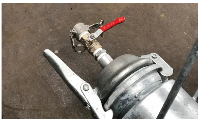
STEP 10: Take one end cap and attach the valve and camlock coupling using teflon tape
