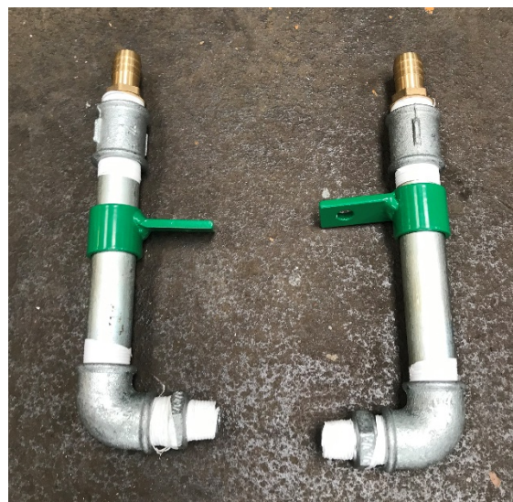
STEP 2: Assemble the suction inlet and pressure outlet using teflon tape
