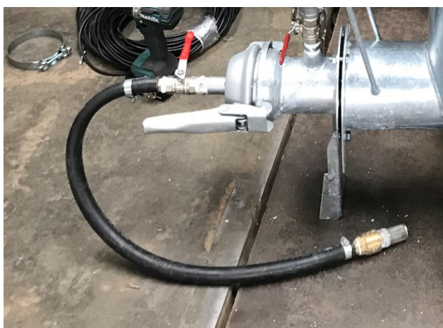
STEP 11: The water hose can now be connected to the valve with a nipple and hose clamp. Attach on the end of the hose the non-return valve
