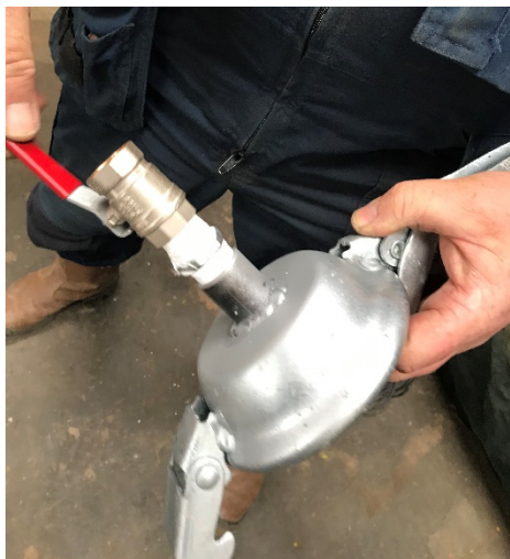
STEP 10: Take one end cap and attach the valve and camlock coupling using teflon tape
