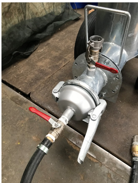
STEP 11: The water hose can now be connected to the valve with a nipple and hose clamp. Attach on the end of the hose the non-return valve
