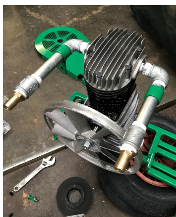
STEP 3: Fix the engine on the frame with bolts and nuts and add the pulley with the key and taper bush
