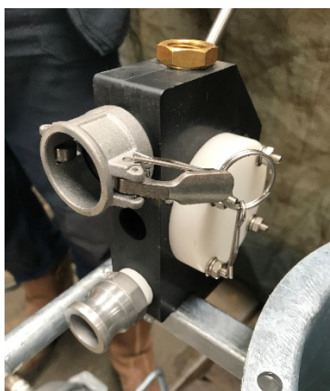
STEP 12: Add the control block, fix it using the long bolt and nut. Add female and male camlocks with teflon tape
