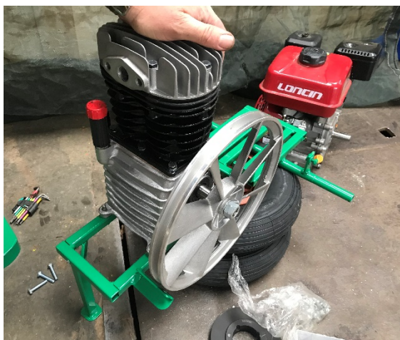
STEP 1: Place the compressor on the frame and attach it with the bolts and nuts
