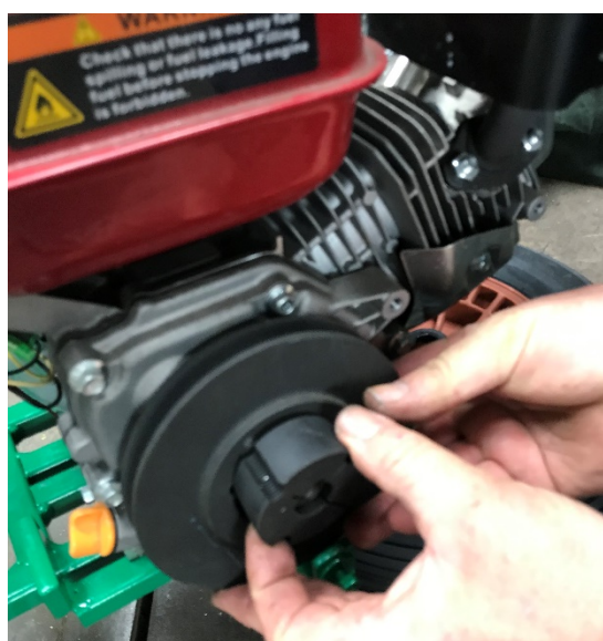
STEP 3: Fix the engine on the frame with bolts and nuts and add the pulley with the key and taper bush
