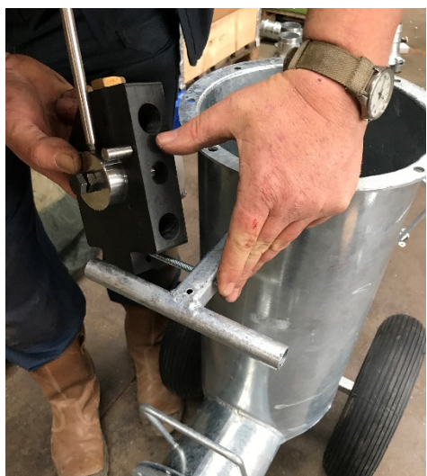
STEP 12: Add the control block, fix it using the long bolt and nut. Add female and male camlocks with teflon tape
