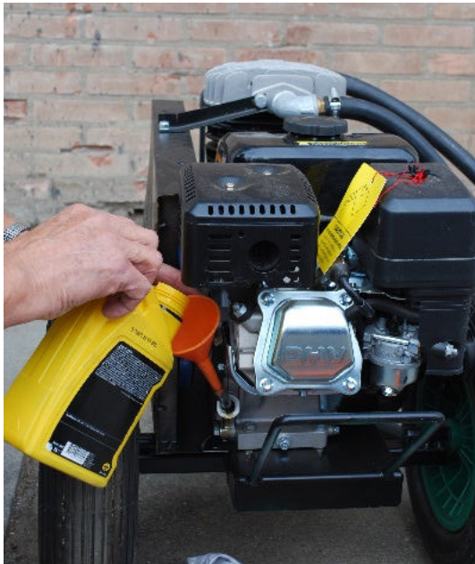
STEP 2: Fill engine and compressor with oil (10W40) .
