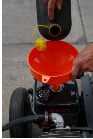
STEP 2: Fill engine and compressor with oil (10W40) .
